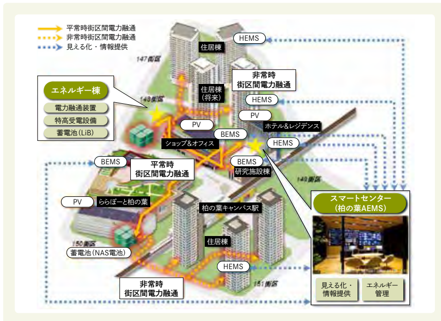
AEMS (Area Energy Management System), BEMS (Building Energy Management System), HEMS (Home Energy Management System), PV (Photovoltaics), LiB (Lithium-ion Battery)
