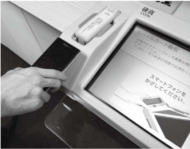
Fig. 2—Using a Mobile Cash Card with an ATM. The ATM is reading the cash card information stored on the smartphone.
