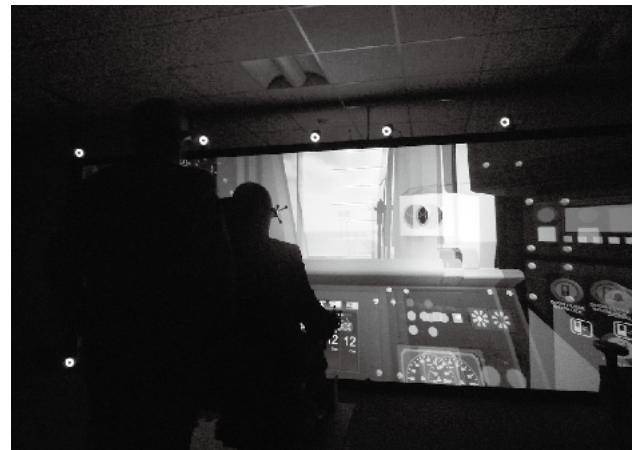
Fig. 7—Virtual Mock-up of Driving Cab Area. The photo shows a customer review being conducted using screen projection virtual reality at the Virtual Engineering Centre of the University of Liverpool.
