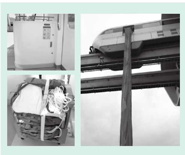
Fig. 7—Passenger Evacuation Equipment. Spiral chutes are located in boxes (top left) behind the viewing seats in the front and rear cars, and are used by opening the lid of the box, taking off the cover, and removing them (bottom left). The frame is fixed to a side door and the chute is lowered to the ground (right) to allow passengers to evacuate the train.
