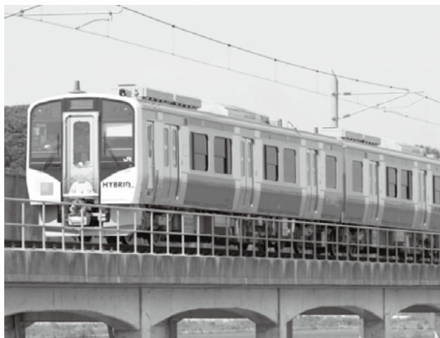
Fig. 6—Series HB-E210 Train. A new series was introduced to enable through services between DC and AC line sections.
