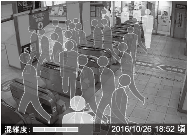
Fig. 6—Eki-Shi-Vision, Tokyu Dentetsu’s Mobile App-based Information Service. The service displays icons overlapping the positions of people in an image to provide intuitive station congestion information while respecting privacy.
