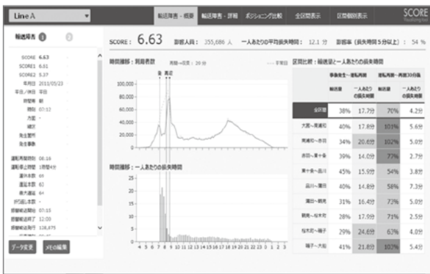
Fig. 4—SCORE System (Joint Study with JR East). The system quantitatively expresses the effect of transportation problems on passengers.
