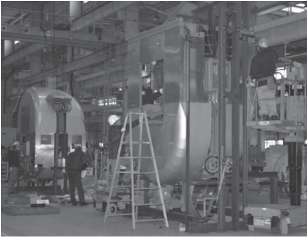
Fig. 18—Assembly of Complete Elevator Car. The photograph shows the trial assembly of a complete elevator car at Mito Works together with construction site workers.
