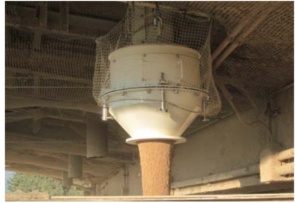
11 State of grain being discharged from a dustless chute
