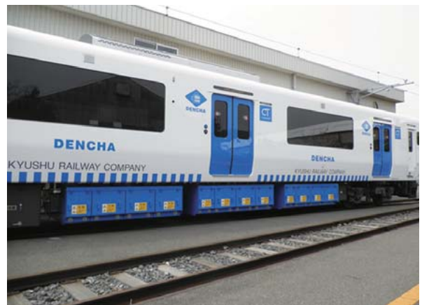
7 AC BEMU (top) and main circuit storage battery (bottom)
