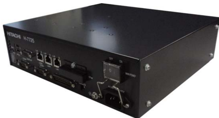
1 Small-sized embedded computer (I/O extended model)
