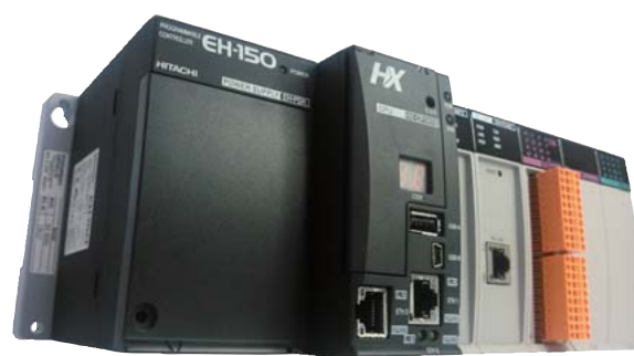
7 Example of HX series configuration combined with I/O module
