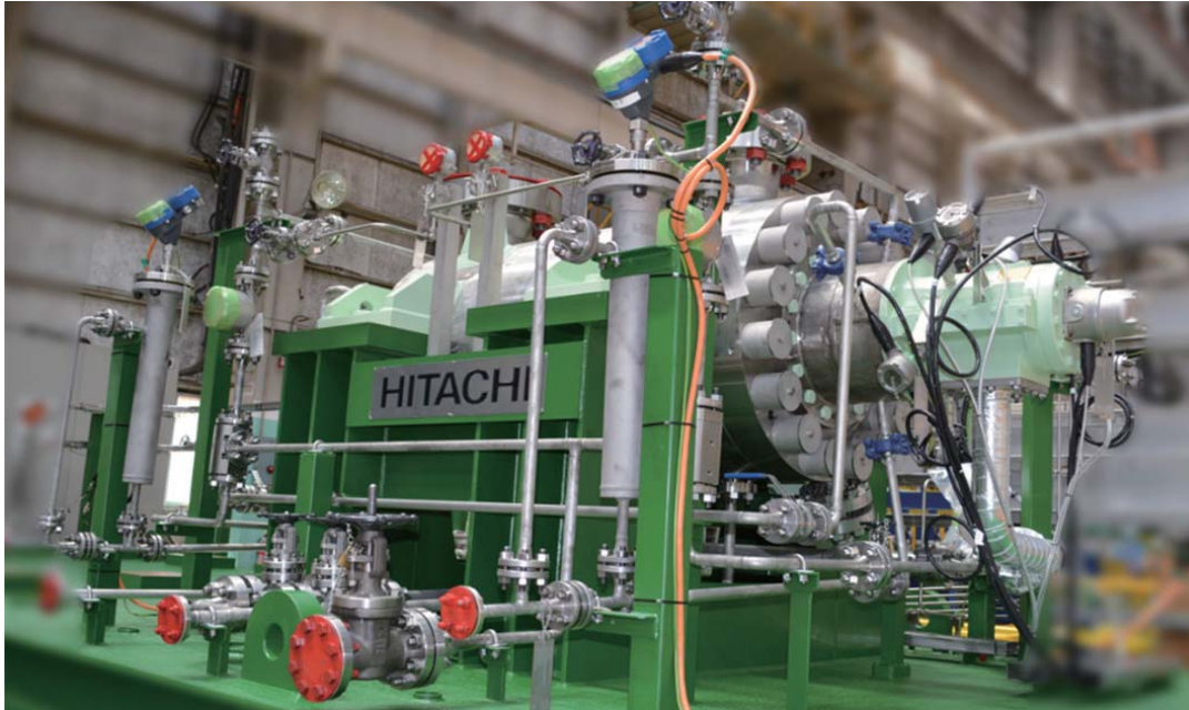
1 Medium-capacity injection pump
