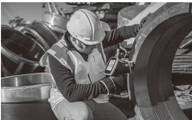
Figure 5 — VULCAN Handheld LIBS Analyzer in Use at Scrap Yard Rapid and accurate analysis is needed to analyze and identify large quantities of scrap metal of different types. The LIBS analyzer is able, for example, to identify the grade of an aluminum alloy in just a few seconds. As the measurement data is managed in the cloud on EXTPOE Connect, users in the field can focus on taking measurements.
