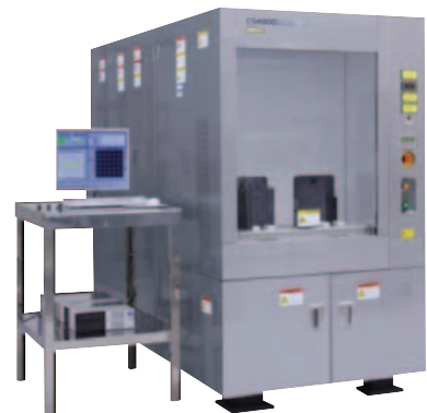
3 CS4800 critical dimension scanning electron microscope (CD-SEM) supporting small-diameter wafers for semiconductors for mass-production of a wide variety of semiconductors
