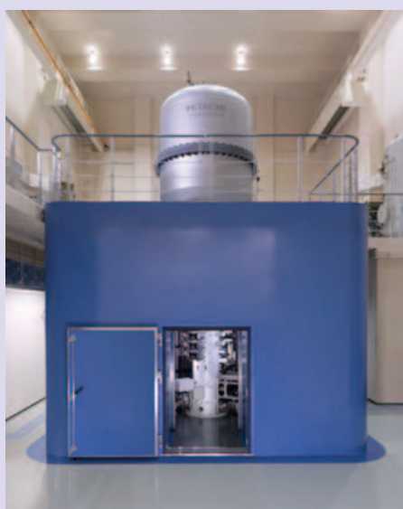
5 Successful observation of distribution of magnetic fields inside a material with world-leading resolution (top) and the atomic-resolution holography electron microscope used for the observations (bottom)
