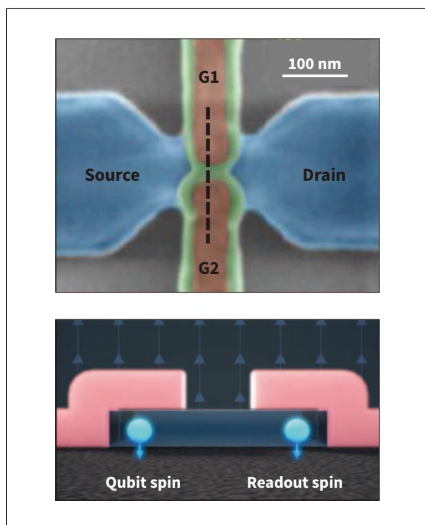
precision on a timescale of approximately 1  $\mu$ s, two orders of magnitude faster than competing techniques, while still retaining the scalability provided by split-gate technology<sup>(4), (5)</sup>. HCL calls this method “gate-based sensing.” Other groups working in the field are adapting the method to their different technologies<sup>(6)</sup>.
